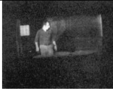
Shorter exposures (e.g., 1/125) capture only part of the raster.
